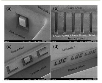
Fig. 3 Water-assisted fs-laser direct-write ablated micropatterns formed on the 500 µm-high sidewall surface of an open microreservoir. 45°-tilted SEM images of (a) an O-shaped pattern and (b) five vertical grooves formed with different writing speeds; (c) 30°-tilted SEM image of an ablated "LOC" logo; (d) 45°-tilted SEM image of ablated "LOC" logos with different sizes and volumes
