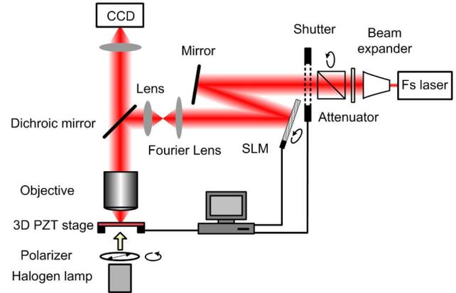
Fig. 1. Optical configuration for holographic recording and reading.
