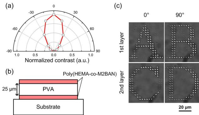
Fig. 4. (a) Readout bits contrast versus the angle between recording and reading polarization. (b) The structure of the storage medium. (c) Readout results of the two-layer polarization-multiplexed data.
