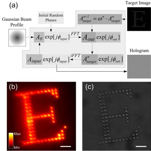
Fig. 2. (a) Flowchart of the weighted GS algorithm. (b) The intensity distribution map of the resulting multiple foci pattern. (c) Recorded bits by a single-shot of femtosecond laser. Scale bar: 10  $\mu\text{m}$ .
