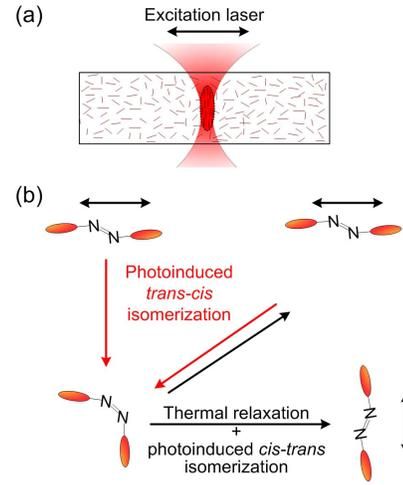
Fig. 3. (a) Photoinduced reorientation of the bisazobenzene molecules. (b) The detailed process of photoinduced isomeric orientation.
